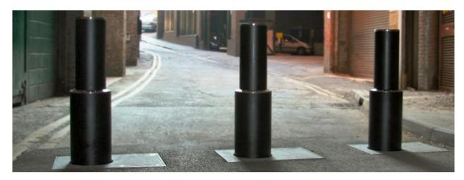
The ATG Access SP Shallow TT has a unique double action retractable design which ensures smooth operation and acts as a depth saving feature. It has been successfully impact tested in accordance with BSI PAS 68:2010, arresting a 7,500kg truck at 64km/h (40mph) and with less than 1m penetration. The SP Shallow TT is the strongest reduced-depth Automatic bollard on the market.
