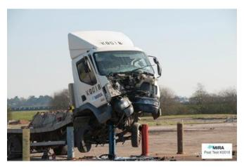
The ATG Access Rapid Deployable Surface Mount Bollard is the world's first impact tested surface mounted bollard system, providing PAS68 certified impact protection.
