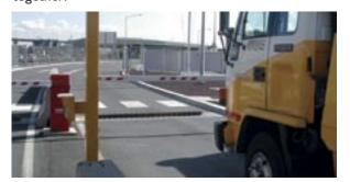
Tyre Spike installations require a boom gate or other traffic signalling device to work in conjunction with the tyre spikes to ensure that the driver knows when it is safe to proceed.
