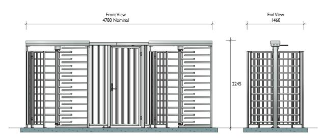
Leda full height turnstiles integrate with other access control systems and cater for a flow of up to 20 people per minute. Controllers can be configured to provide a range of functions (entry only / exit only / entry and exit). Recommended minimum for all concrete footings, 30MPa.
