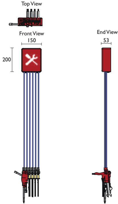
Standard tool kits are fitted to plastic coated steel cables.
