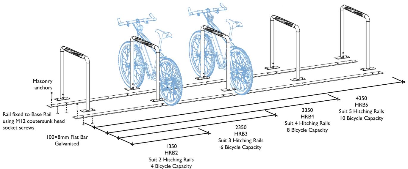
Bicycle rails should be installed at 1000 centres to conform to AS2890.3 requirements allowing easy access for cyclists.
