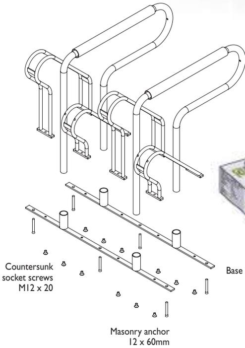
Countersunk socket screws M12 x 20
