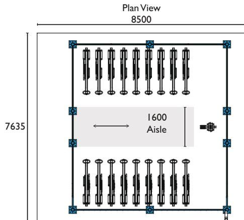
The Palm Cove is a modular design that can be expanded using 1500mm wide panels
