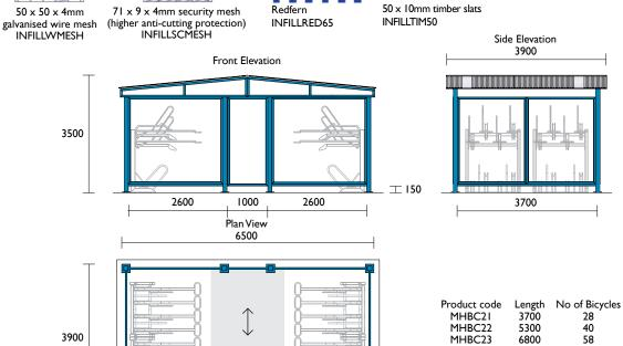
$\begin{tabular}{ll} \textbf{Material Specifications (General)} \\ \textbf{Structure} \\ \textbf{Cladding} \\ \begin{tabular}{ll} 100 \times 100 / 100 \times 50 \text{ steel sections / Galvanised / Powder coated in a range of colours} \\ \textbf{S0} \times 50 \times 4mm / 71 \times 9 \times 4mm \text{ steel mesh / Metal cladding / Galvanised / Powder coated in a range of colours} \\ \end{tabular}$
