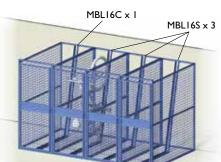
Material Specifications (General) MBL16S/C 25 x 25 x 1.6mm SHS /  $25\times25\times1.6$ mm SHS /  $50\times50\times4$ mm steel mesh / Galvanised / Powder coated in a range of colours Wheel rail, vandal-proof lock, 3-way locking, optional back & roof panels
